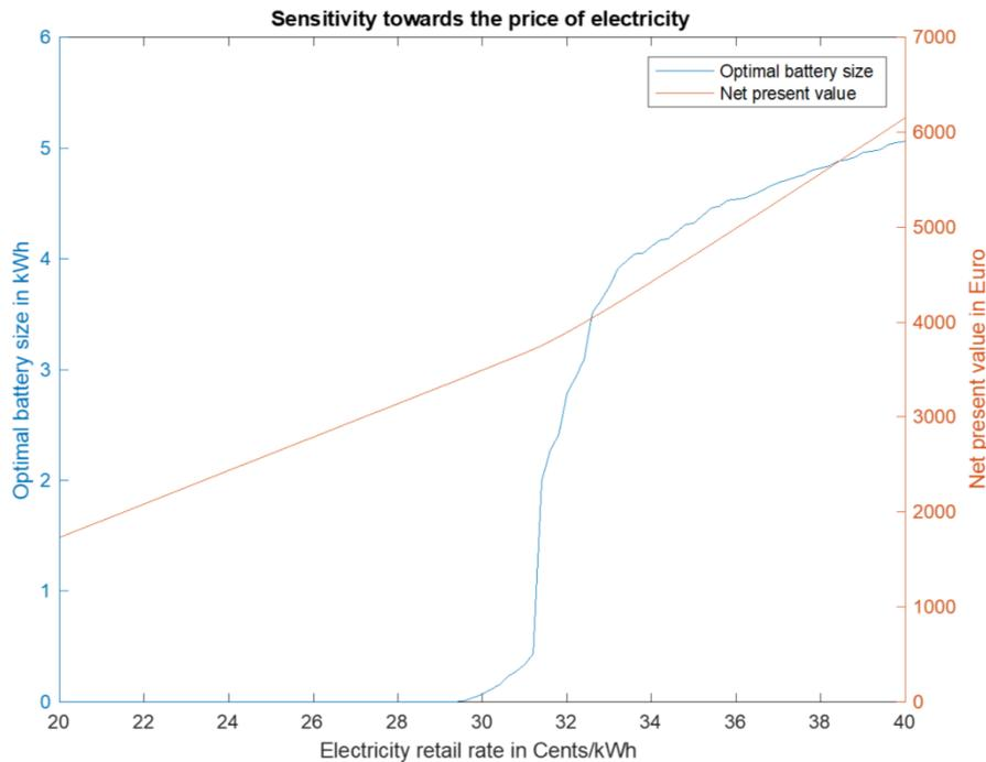
**Figure 16:** Return maximizing battery sizes at different electricity retail rates.
