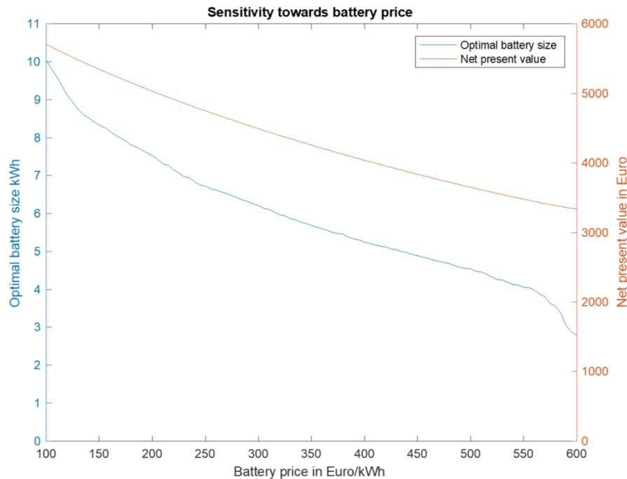
Figure 19: Return-maximizing battery sizes in a "2020 scenario".
