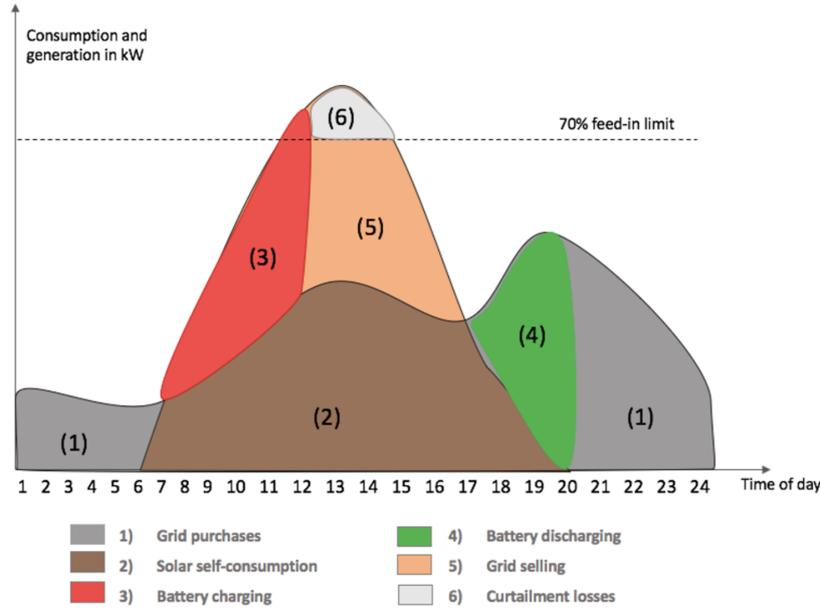
**Figure 3:** Model for daily pattern of photovoltaic generation and consumption.
