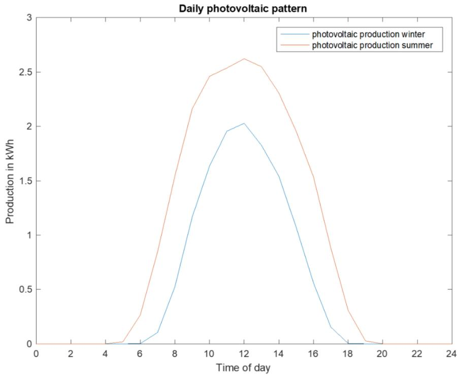
**Figure 8:** Daily production pattern of the photovoltaic system in winter and summer.
