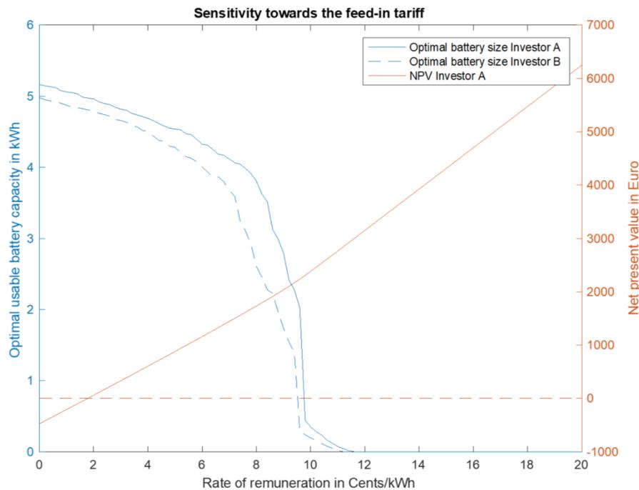
**Figure 17:** Return-maximizing battery sizes for different feed-in tariffs.
