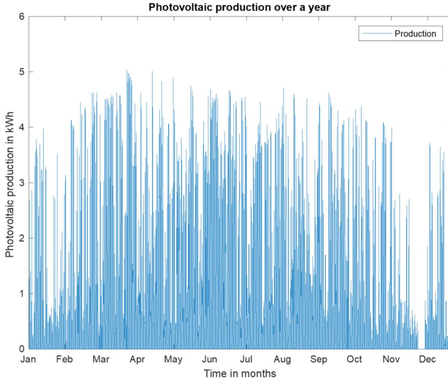
**Figure 7:** Hourly photovoltaic generation over a year.
