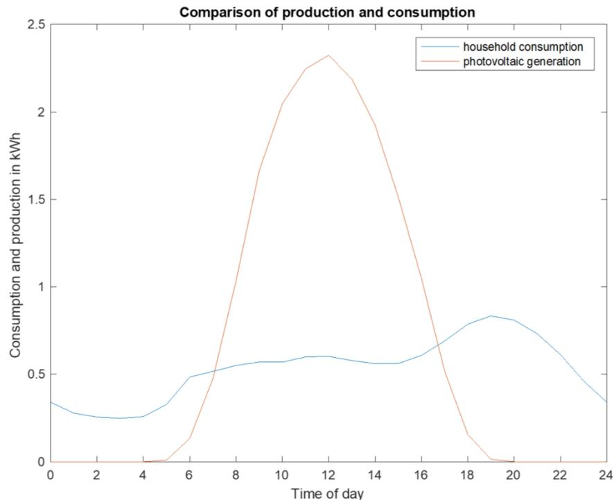
**Figure 14:** Comparison of the daily consumption and production pattern.
