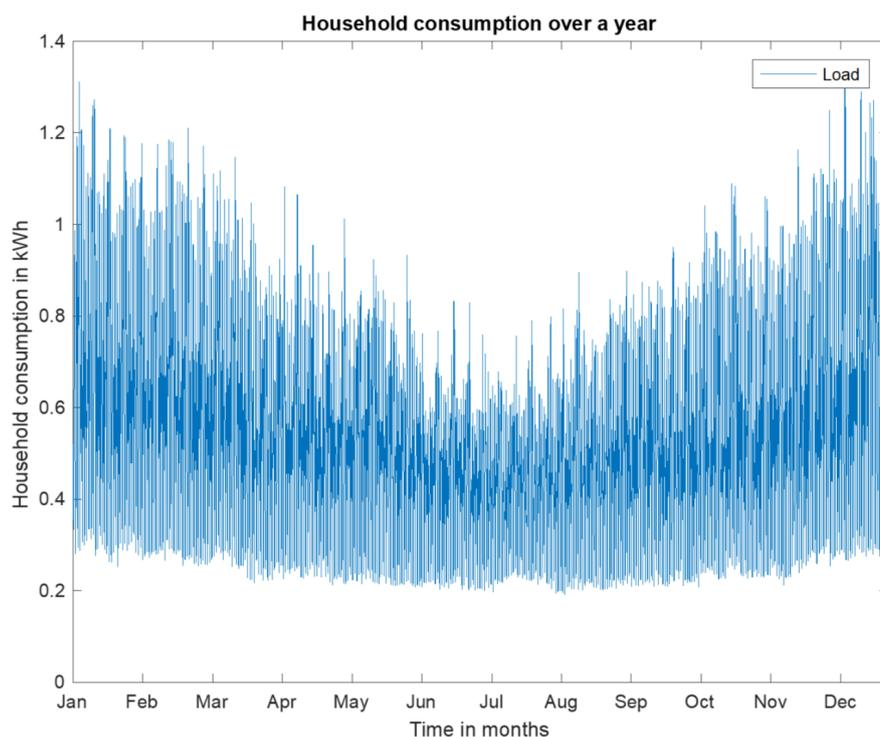
**Figure 5:** Load profile of an average household in hourly steps over a year. (Based on analysis of data from Berlin (2015).)
