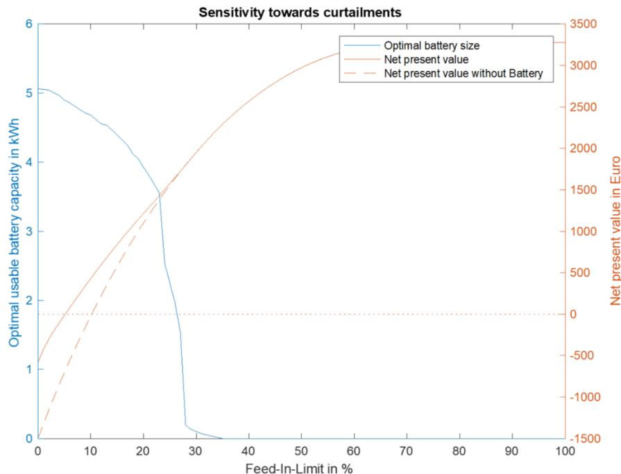
**Figure 18:** Return-maximizing battery sizes at different feed-in limit regulations.
